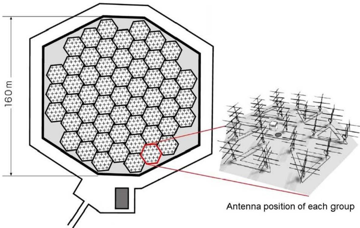
**Figure 5:** The EMU radar antenna array. Each cross represents the location of a three-element Yagi antenna and TR module.
