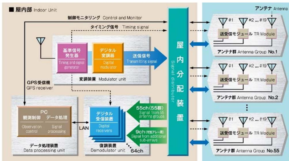
**Figure 6:** Schematic diagram of the EMU radar.
