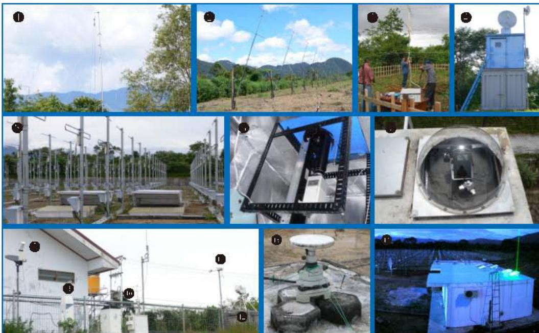
**Figure 3:** Equipment installed at the Equatorial Atmosphere Observatory. (1: FM-CW ionosonde, 2: VHF radar, 3: Meteor radar, 4: X-band meteorological radar, 5: RASS speakers, 6: All-sky imager, 7: Fabry-Perot interferometer, 8: Micro-rain radar, 9: Ceilometer, 10: Disdrometer, 11: Optical rain gauge, 12: Radiometer, 13: GPS receiver, 14: Lidar)
