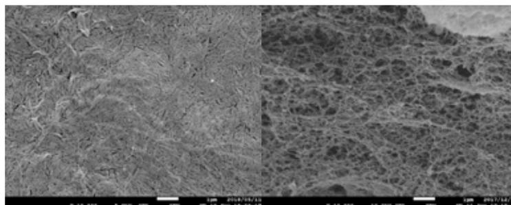
Figure 1. SEM images of cellulose nanofibers disintegrated by mechanical treatment in water with (left) and without (right) sericin after supercritical CO<sub>2</sub> extraction
