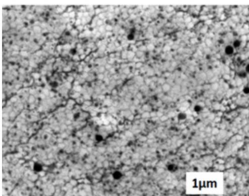
Figure 1. CNF-acrylic resin composite.
