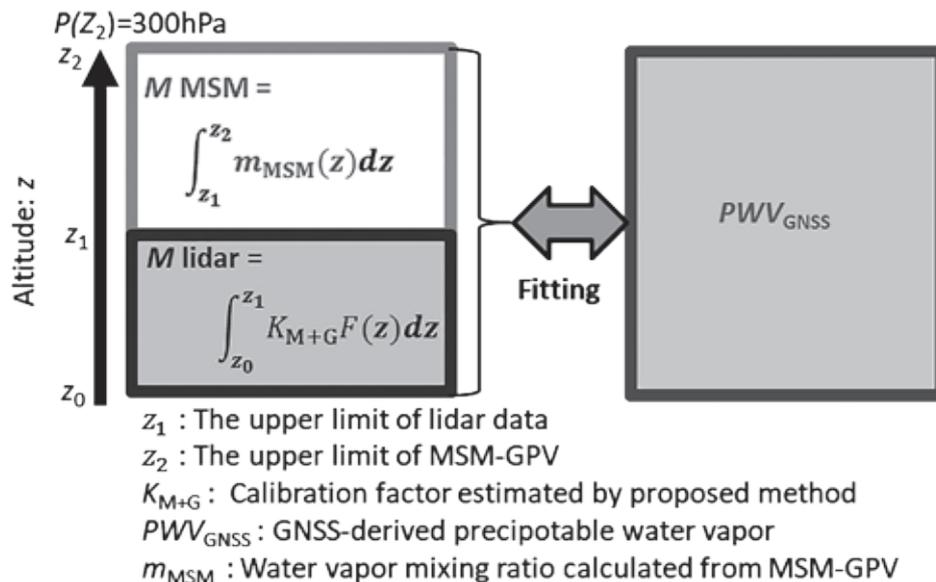
Figure 1. Schematic of new Raman lidar calibration method using GNSS-PWV and MSM. The function  $F(z)$  indicates the relative water vapor profile calculated from the Raman lidar signals for each molecule. The calibration factor  $K_{\text{M+G}}$  is estimated by fitting the GNSS-PWV to integrated water vapor profiles combined with the MSM and the results of the Raman lidar observation.
