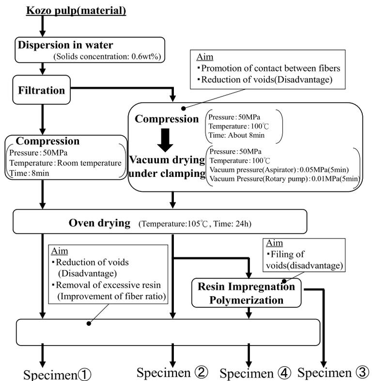
Figure 1. Manufacturing procedure
