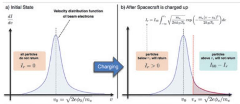
Fig.1: A new returning current model for active spacecraft charging.
