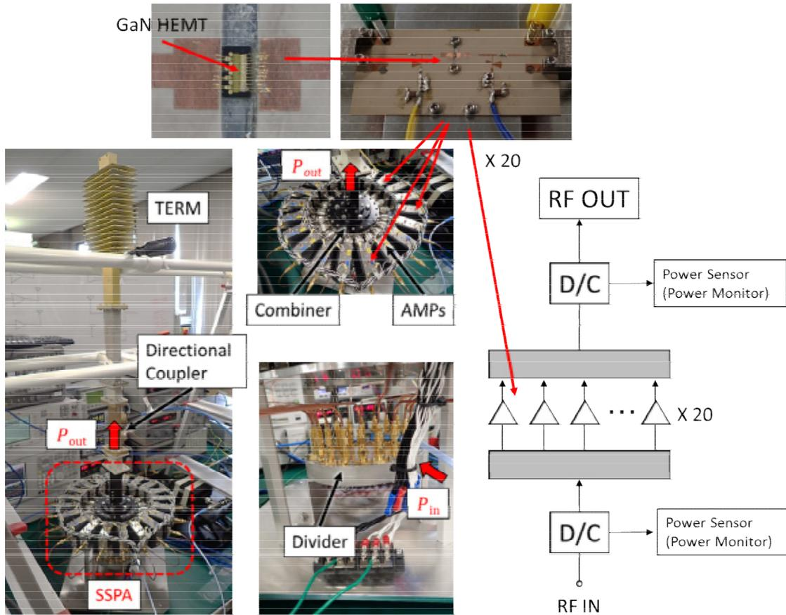
Fig.1: Developed 20-Combined C-band GaN amplifier (179.8 W).
