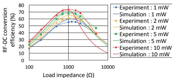
Figure 3. Experimental result of the rectifier with continuous input.
