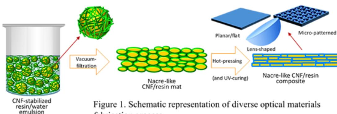
Figure 1. Schematic representation of diverse optical materials fabrication process.
