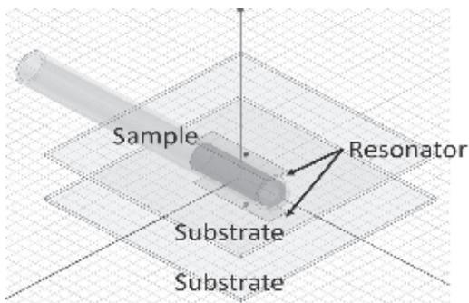
Figure 1. Simulation model of a heating device using broad side coupling
