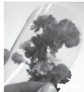
Figure 1. Wood pulp-based optically transparent nanocomposite.
