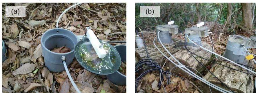
Fig. 1. Automated chamber for measurement of CO<sub>2</sub> efflux from (a) leaf litter and (b) coarse woody debris
