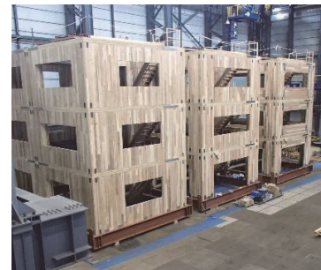
Figure 3. Shaking table test
