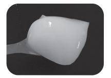
Figure 1. Appearance of 8 % cellulose nanofiber suspension in 8 % NaOH solution.
