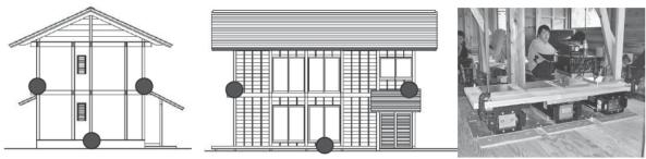
Figure 1. Locations of velocity meters and feature of excitation test on the second floor.
