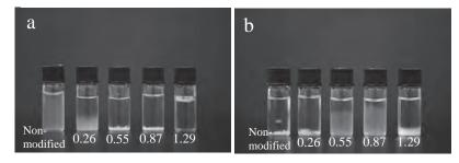
Figure 2. Dispersibilty of octanoylated CNF in water (a) and hexane (b).
