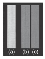
Figure 1. Untreated specimen as control (a), colored specimens during natural aging for approx. 1600 years (b) and heated at 180°C for 12 hours (c).
