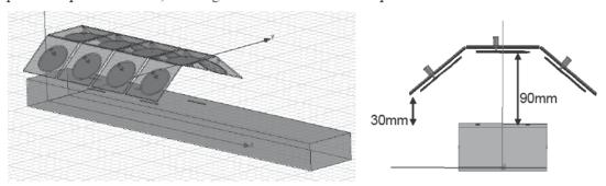
Figure 1. Oblique receiving unit (rectenna) which increases the transmitting efficiency of 84.4%
