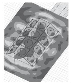
Figure 2. Simulation result of microwave propagation between transmitting and receiving antenna.
