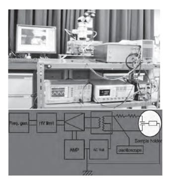
Figure 1 A general experimental setup.
