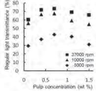
Figure 2. The regular light transmittance at 600 nm of 15 composites made of acrylic resin and 10 min agitated pulp at various agitating speed for pulp suspension of 0.1, 0.4, 0.7, 1.1 and 1.5 wt%.
