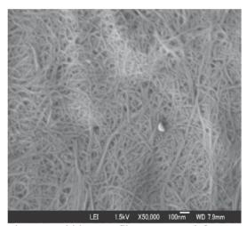
Figure 1. chitin nanofibers extracted from crab shells via high-speed blender under acidic conditions (pH 3-4)
