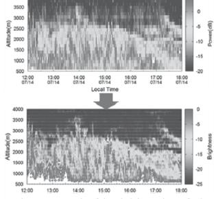
Figure 2. Example of time-height sections of echo intensities observed with standard mode (upper) and FDI mode (lower) of LO-7.
