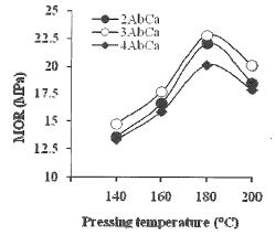
Fig 2. Tensile strength of molded products made from acacia bark (Ab) reinforced with citric acid (Ca) and pressed on 4 MPa for 10 mins. 2AbCa = 33.33% of Ca; 3AbCa = 25% of Ca and 4AbCa = 20% of Ca.
