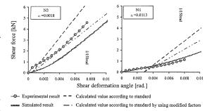
Figure 2. Example of simulated and experimental results on shearing of lattice shear wall.
