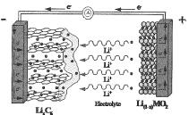
Figure 1. Electrode reactions in lithium ion cells.
