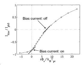
Figure 1. The voltage-current characteristic curve obtained by changing the magnitude of the bias current. The zero potential corresponds to the background space potential.
