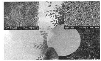
Figure 1. Optically transparent nanofiber paper (left) composed of 15nm cellulose nanofibers (upper left, scale bar in inset: 100 nm) and conventional cellulose paper (right) composed of 30 um pulp fibers (upper right, scale bar in inset: 200µm).
