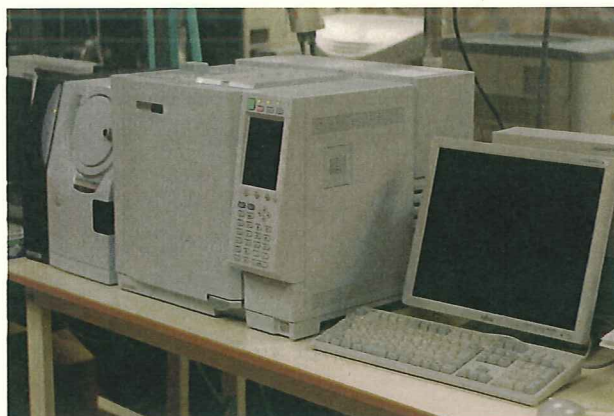
A "Shimadzu GCMS QP-2010 Plus" unit used for kinetic analysis of the recombinant proteins
