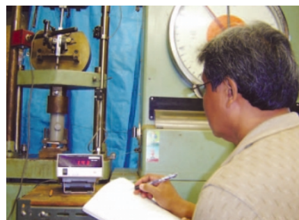
Compressing of wood samples for penetrability and recovery test
