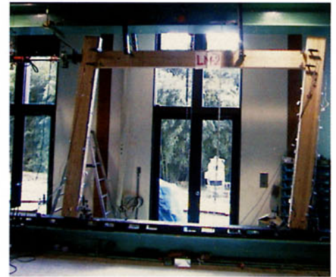
An image of the portal frame made of LVL subjected to a push-pull cyclic lateral loading for evaluating structural performance of beam-column joints. (Photo. 2)
