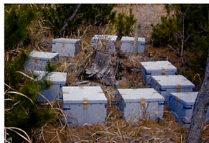
Field test for wood degradation at a site infested with termites
