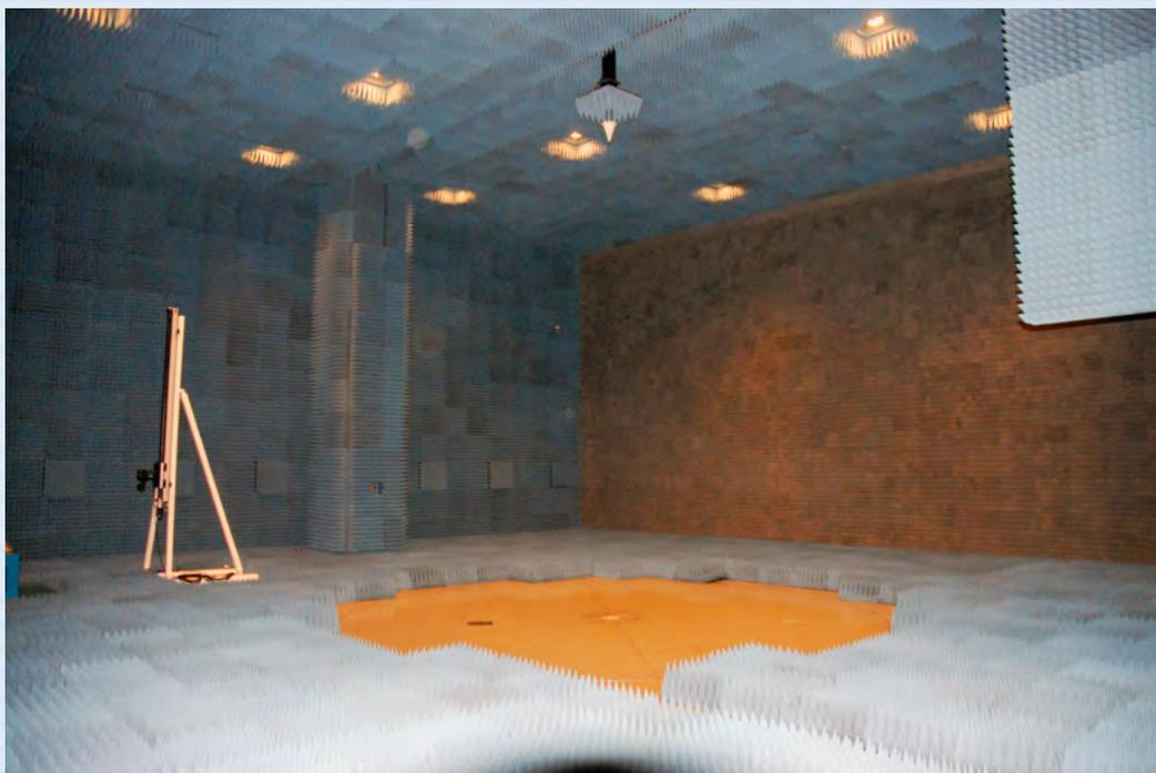
SPSLAB is a research laboratory with a plane-type, near-field scanner in a shielded room for taking  $3 \text{ m} \times 3 \text{ m}$  antenna measurements. This allows for the design, development, measurement, and analysis of antennas and microwave circuits.
