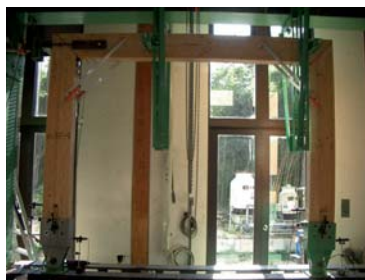
Lateral shear test on a glulam portal frame
