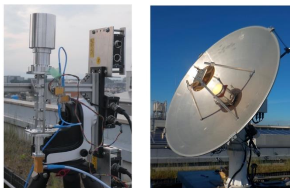
16 - 64 GHz wideband feed under developing for the radiometer(left), and 2.4 m antenna(Right) of NICT with 3.2 - 16 GHz wideband feed for VLBI, which will be used for the radiometer with new feed.
