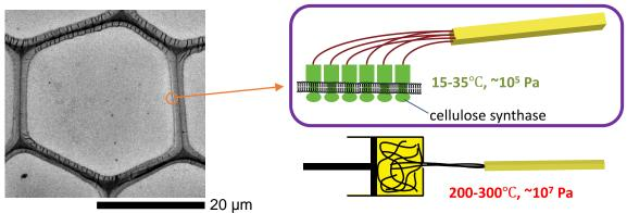
Wood is polymer composite and its synthesis is done by enzyme protein at ambient temperature and pressure in aqueous environment. This synthetic condition is eco-friendly in comparison with the case of a synthetic polymer like polypropylene.
