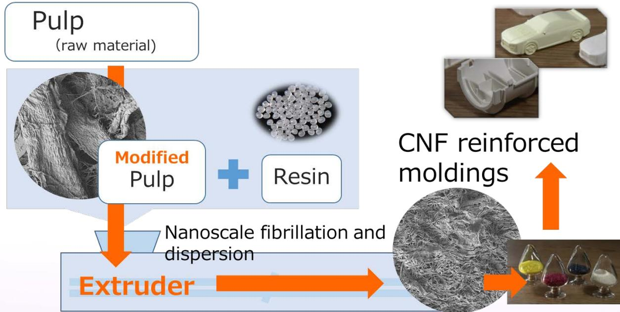
Pulp direct kneading method "Kyoto Process"
