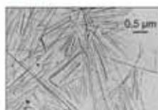
Monocrystalline cellulose domains parallel to the microfibril axis composed of cellulose chains in a cellulose lattice bonded laterally and surrounded by surface chains forming a pentacrystalline amorphous
