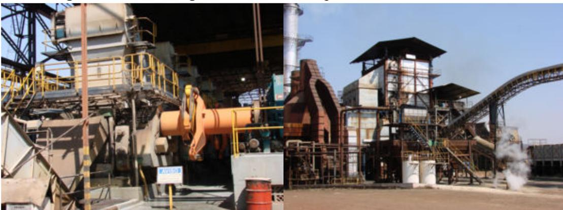
**Fig. 6** Left: steam turbine driven mills. Right: boiler.
