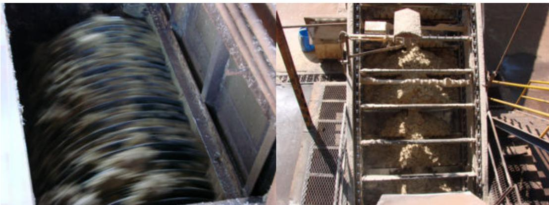
**Fig. 4** Left: sugar cane being squeezed in the mill. Right: sugar cane bagasse ready to feed the boilers.
