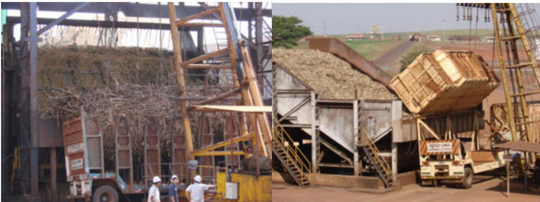
**Fig. 2** Left: whole canes being fed by hillo-type crane. Right: chopped cane being unloaded.
