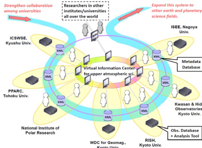
**Figure 8:** Schematic view of the virtual information center of the IUGONET project. A metadata database is distributed at the IUGONET institutes, as shown with boxes labeled “XML”, and connected to other metadata databases through the Internet in order to share all the metadata. In addition, data analysis software to handle various kinds of solar-terrestrial environment observation data is developed (Modified from Hayashi et al [2013]).
