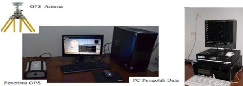
Figure 2. GPS Ionospheric Scintillation and TEC Monitor (Left) and Ionosonde (Right)
