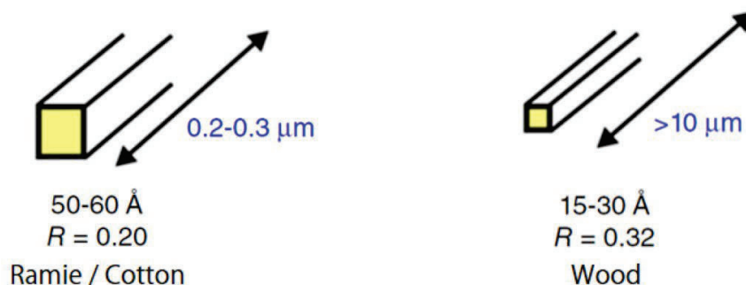
Fig. 10. Different crystallite sizes for cellulose from different sources. R stands for the ratio of surface chains to total chains.
