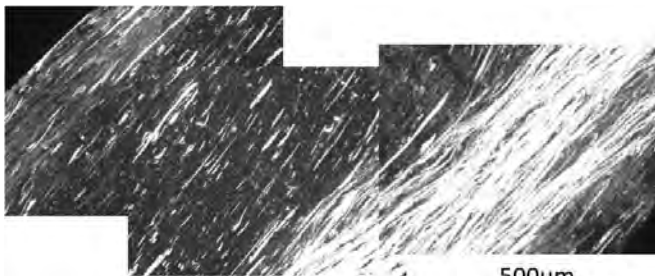
PE/変性CNF10%+膨潤-140°C混練 (3100, 53.9)
