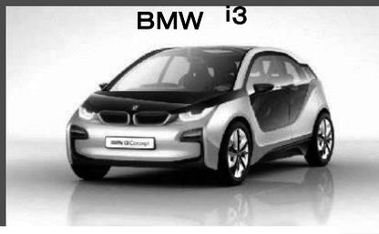
CFRP Body (HP-RTM molding)
