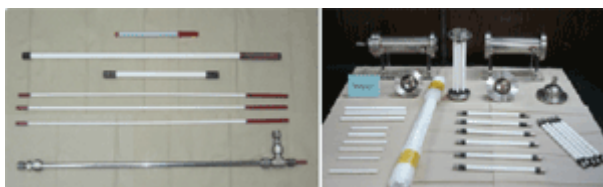
Ceramic membranes and their module for mid-temperature carbon dioxide separation
