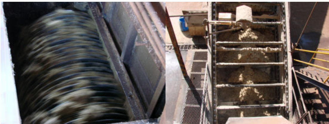
Fig. 4 Left: sugar cane being squeezed in the mill. Right: sugar cane bagasse ready to feed the boilers.
