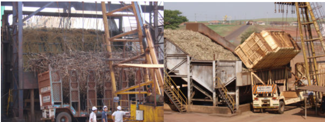
Fig. 2 Left: whole canes being fed by hillo-type crane. Right: chopped cane being unloaded.
