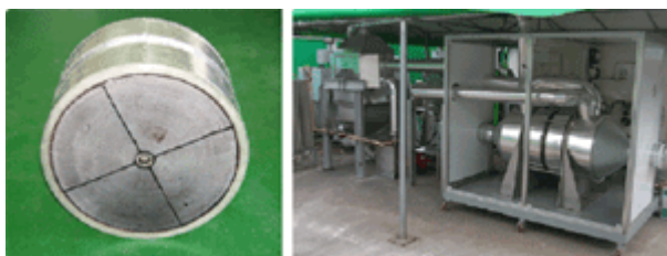
Adsorptive honeycomb rotor and TSA system for VOC concentration
