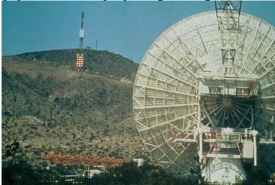
Fig. A.2.1. Microwave power transmission over 1.54km
