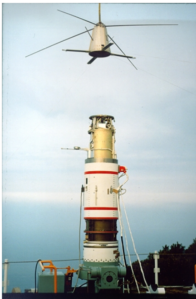
Fig. A.4.1 MINIX, the world-first MPT experiment in the ionosphere. ©RISH, Kyoto University
