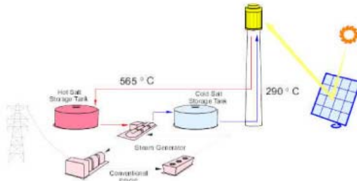
Figure E.5.2: Outline of a terrestrial solar tower plant
