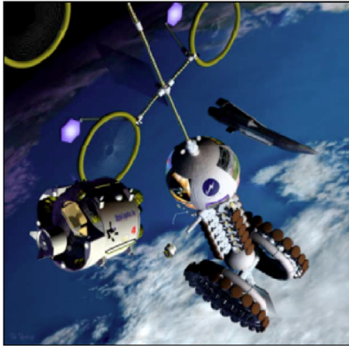
Figure C.9.2. A Space Business Park concept for a multipurpose commercial space station with artificial-g spinning ring, zero-g staterooms, and an inflatable arena sphere
