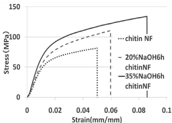
Figure 1. Stress-strain curves of surface deacetylated chitin nanofiber sheet.
