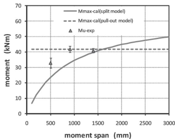
Figure. Test results of loading test on the joints and calculation for moment and moment span
