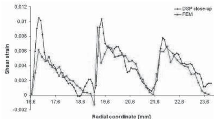
Figure 2. Shear strain profiles. Experimental DSP shear strain measurements and predicted shear strain using finite element analysis.
