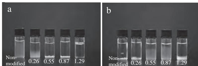
Figure 2. Dispersibility of octanoylated CNF in water (a) and hexane (b).
