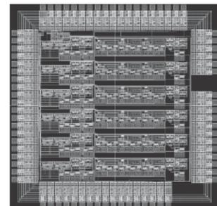
Figure 2. The layout of the waveform receiver.
