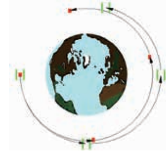
Figure 2 A schematic view of an orbiting drop tower experiment (quoted from http://einstein.stanford.edu/STEP/ ; not drawn to scale). A pair of test masses, made of different materials, is put in a low Earth orbit (about 500 km above surface); the test masses are in free fall in the Earth's gravitational field. If the universality of free fall were violated, there would be differential acceleration between the test masses, as shown in this schematic figure (not drawn to scale). Any differential acceleration between the test masses is detected by a position sensor (not drawn).
