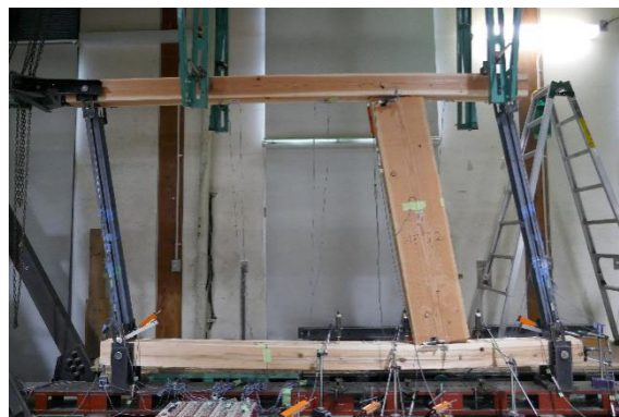
(c) Pull-in side (1/10rad, final stage)
