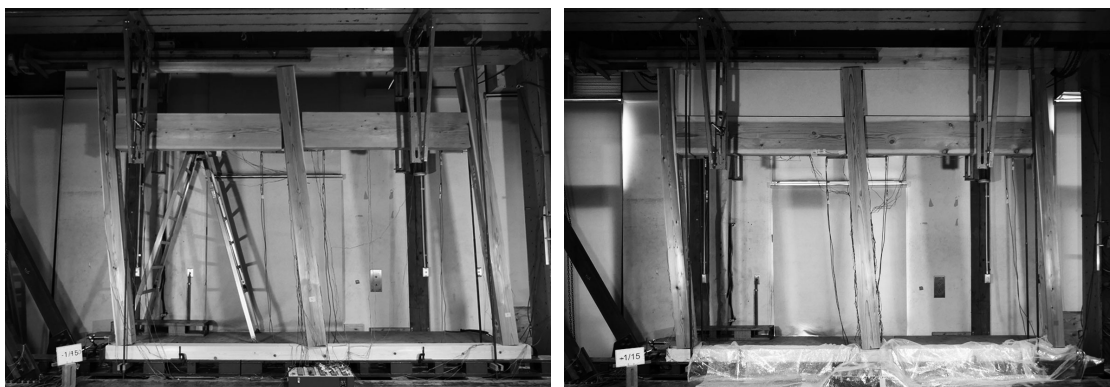
Figure 1. The cyclic loading test of the frame with and without hanging mud wall
