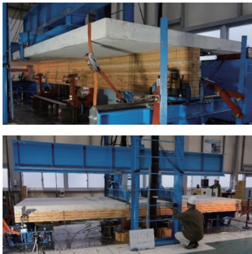
Fig1: Test scene of glulam beam with RC slab (Upper) and CLT with RC slab (Bottom)
