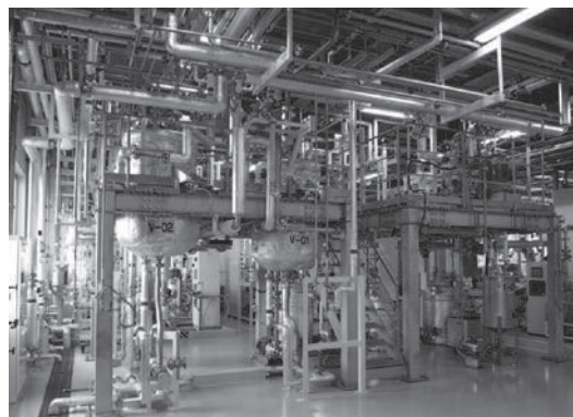
Fig. 1 Bench scale plant for bioethanol production from woody biomass (NEDO project).
