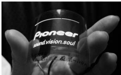
有機EL device emitted on a cellulose nanofiber - resin composite transparent sheet (Yano, 2007)
