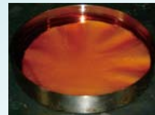
PF resin Impregnation (MW=3,351) at 20°C
