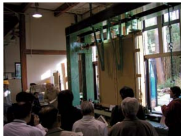
Open experiment for re-evaluation of the traditional Kyoto-style mud shear wall
